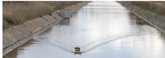
Tests with no bubble injection: two symmetric bow waves on both side of the barge
