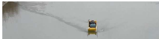
Tests with bubble injection on left board: the bow wave is completely limited by the side fed in compressed air.
