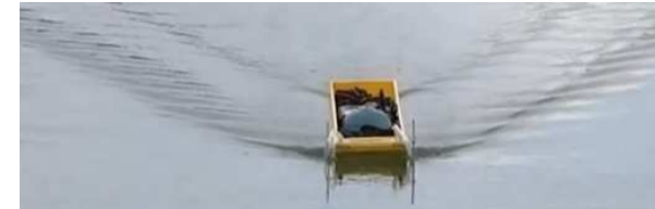
Tests with no bubble injection: two symmetric bow waves on both side of the barge
