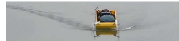
Tests with bubble injection on left board: the bow wave is completely limited by the side fed in compressed air.
