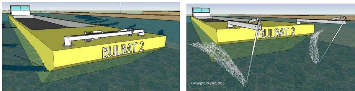
**Figures 7 et 8** : Implementation of the device BULBAT on a river boat
