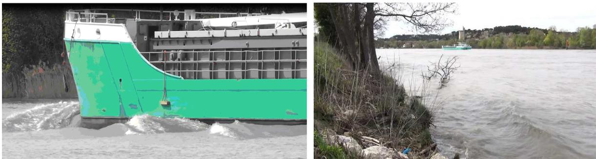
**Figures 2 et 3** : River sea cargo vessel on the Rhône to Villeneuve-lès-Avignon. Waves impacting on banks after the passage of the boat (photos JM. Beynet, in April 3<sup>rd</sup>, 2015)
